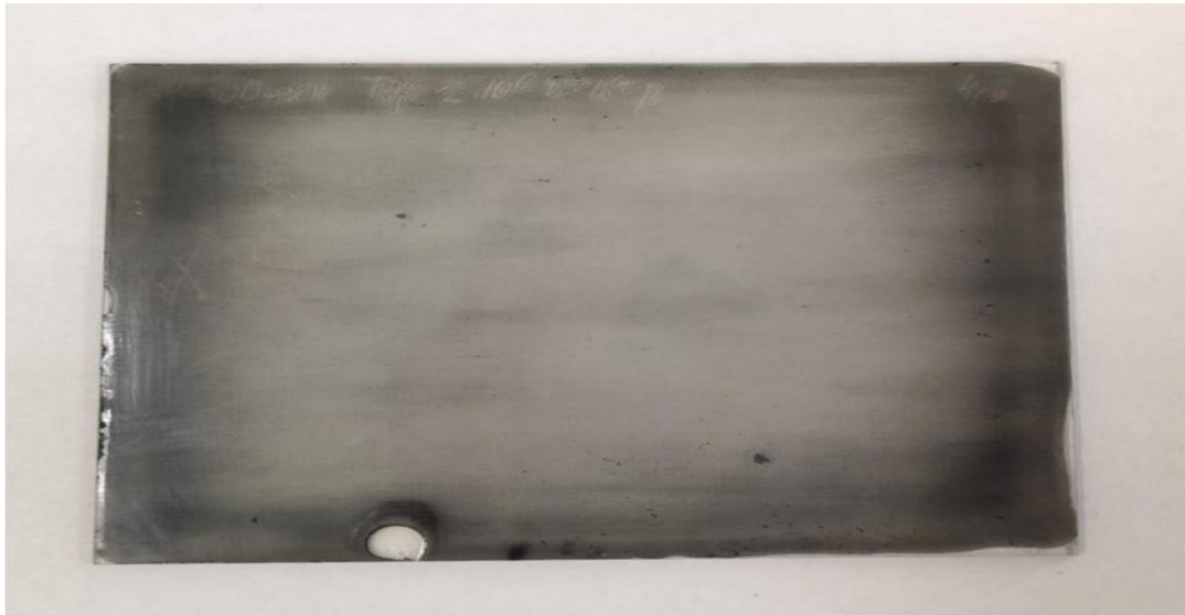
Fig. 1. NTE plate after chemical development. The typical size of NTE plate is 9x12 cm 2 with around 100 mkm thickness of sensitive emulsion layer.
